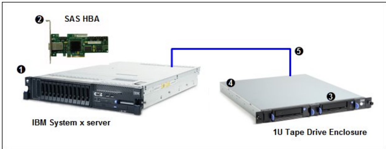
Figure 5. The tape drive installed in an IBM 1U Tape Drive External Enclosure and connected to a System x server
