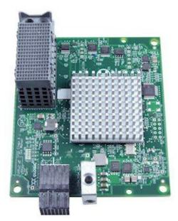
Figure 1. IBM Flex System FC3172 2-port 8Gb FC Adapter
