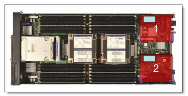
Figure 2. Location of the I/O adapter slots in the IBM Flex System x240 Compute Node
