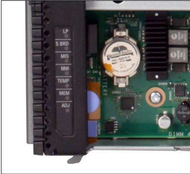
Figure 9. Location of x440 light path diagnostics panel
