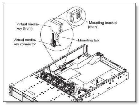
Figure 1. Installing the Virtual Media Key in the IBM System x3620 M3
