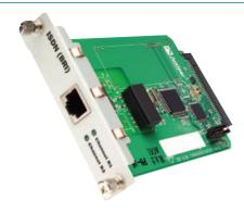
The Juniper Networks single-port ISDN BRI Mini Physical Interface Modules (Mini-PIM) for the SSG 20 platform complements the five on-board 10/100 Ethernet interfaces with expanded WAN connectivity. The ISDN BRI Mini-PIM includes a single physical port supporting ISDN BRI S/T interface types. For ISDN U interface support, an external NT-1 is required.
