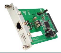
The Juniper Networks optional single-port T1 Mini Physical Interface Modules (Mini-PIM) for the SSG 20 platform complement the five on-board 10/100 Ethernet interfaces with expanded WAN connectivity. The T1 Mini-PIMs include one physical T1 port with an integrated CSU/DSU.
