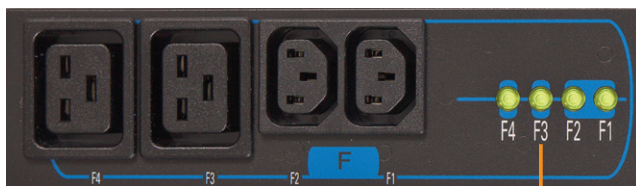
LEDs represent each outlet
