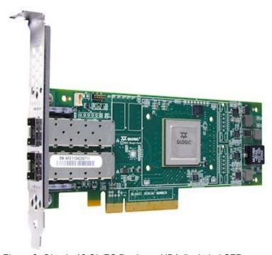
Figure 2. QLogic 16 Gb FC Dual-port HBA (included SFP+ transceivers are not present)
