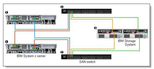
Figure 3. System x server with QLogic 16 Gb FC adapters connected to an external IBM System Storage DS3500 through SAN switches
