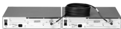
An XRN Distributed Fabric using 3Com Switch 4060s, the XRN Interconnect Kit, and the 5m Interconnect Cable
