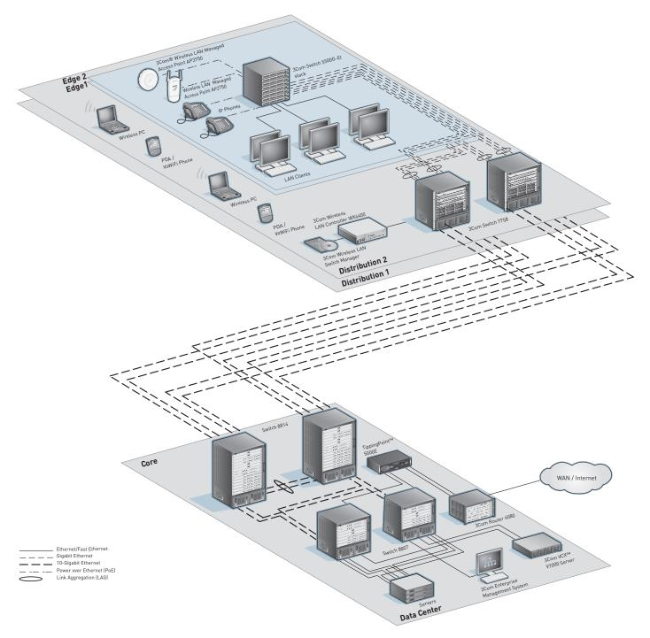
In the above network, 3Com Switch 4500G and Switch 5500G-EI units are managed as a single cluster.
