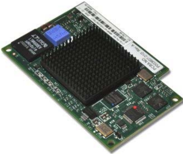
Figure 1. Emulex 8Gb Fibre Channel Expansion Card (CIOv)
