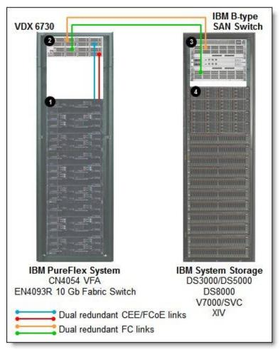
Figure 7. EN4093R as an FCoE transit switch with the Brocade VDX 6730 as an FCF
