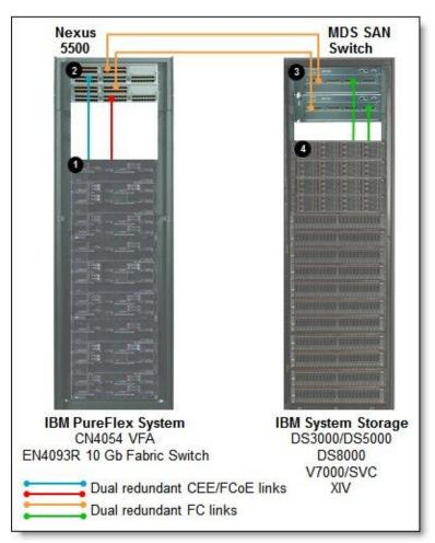
Figure 8. EN4093R as an FCoE transit switch with the Cisco Nexus 5548/5596 as an FCF
