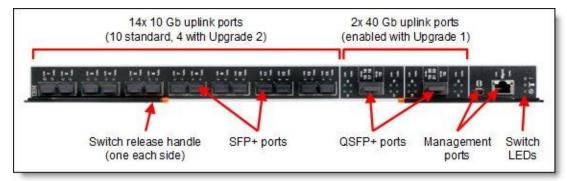
Figure 5. Front panel of the IBM Flex System Fabric EN4093 and EN4093R 10Gb Scalable Switches
