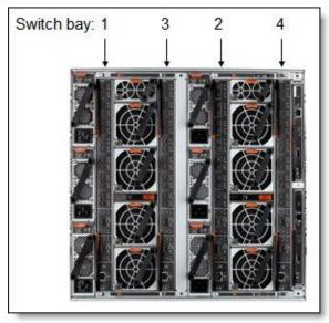
Figure 2. Location of the switch bays in the IBM Flex System Enterprise Chassis
