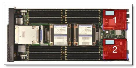
Figure 4. Location of the I/O adapter slots in the IBM Flex System x240 Compute Node
