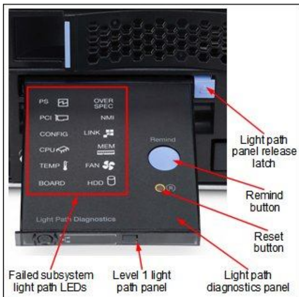
Figure 10. Advanced (level 2) light path for models with eight drive bays
