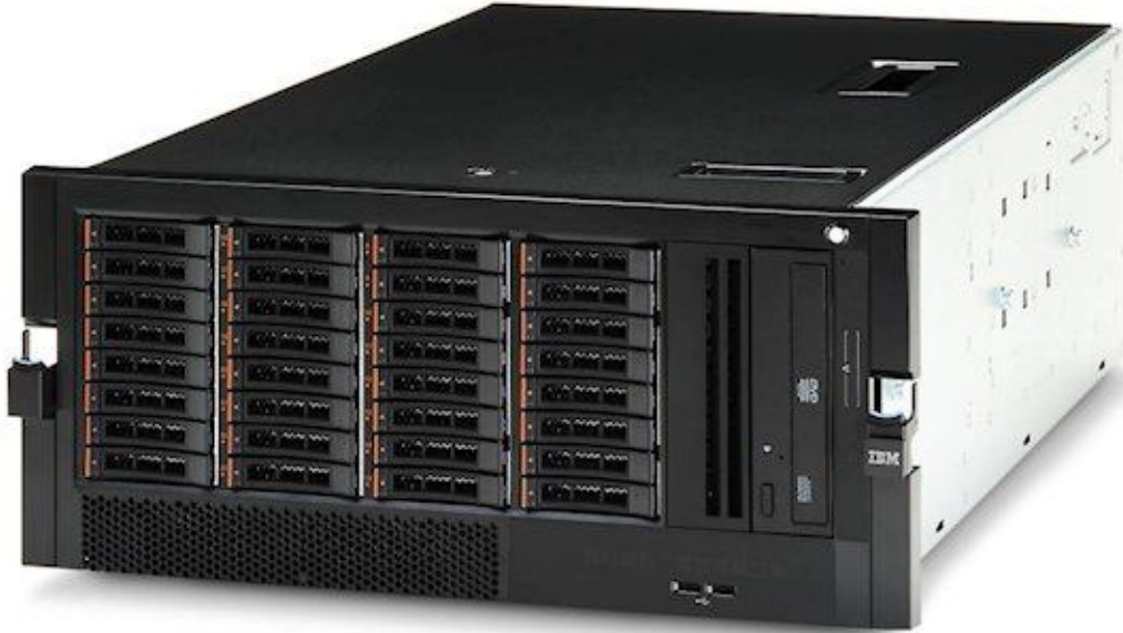
Figure 6. The IBM System x3500 M4 with the Tower to Rack Conversion Kit
