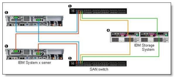
Figure 3. x3650 M3 server with Emulex 16 Gb FC adapters connected to an external IBM System Storage DS3500 through SAN switches
