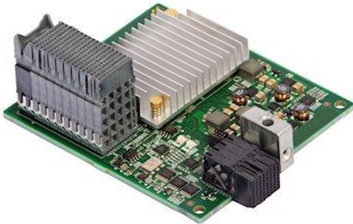
Figure 1. IBM Flex System FC5022 2-port 16Gb FC Adapter
