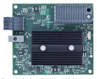
Figure 1. IBM Flex System EN4132 2-port 10Gb Ethernet Adapter
