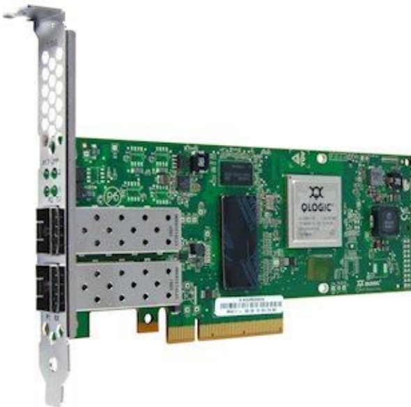
Figure 1. QLogic 8200 Dual Port 10GbE SFP+ VFA for IBM System x
