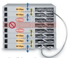
In the unlikely event of a switch failure, the stack integrity is maintained: remaining switches continue to work as a stack.
