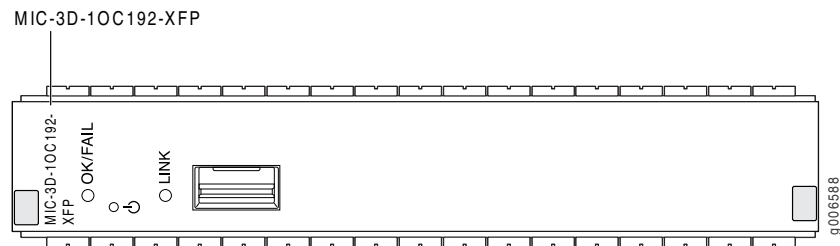
Figure 21: SONET/SDH OC192/STM64 MIC with XFP
