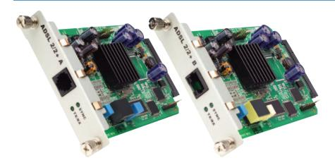
The Juniper Networks ADSL2/2+ Mini-Physical Interface Modules (Mini-PIMs) are for use with the SSG 20 platform. The ADSL2/2+ Mini-PIMs, one supporting Annex A (over POTS) and the other Annex B (over ISDN), each include one physical ADSL port that support ADSL, ADSL2 or ADSL2+ protocols.
